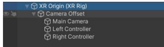
Figure 7: The recommended Hierarchy configuration of the XR origin is the default setting. Please note that "XR origin" refers to both the parent anchor GameObject and the Hierarchy in its entirety.
